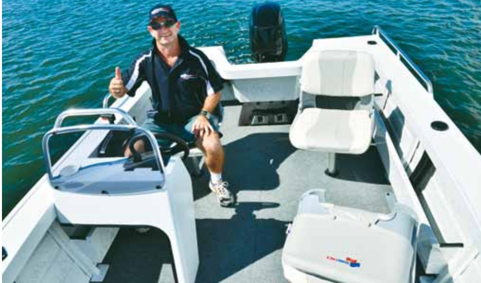
Quintrex's new "Renegade" models are very well fitted out indeed for affordable packages and feature a new stretch-formed variable deadrise hull which looks little different to the average tinny but outperforms them significantly on rough water. Pictured inside and out is the Renegade 460.
