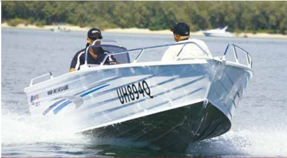
Quintrex's new "Renegade" models are very well fitted out indeed for affordable packages and feature a new stretch-formed variable deadrise hull which looks little different to the average tinny but outperforms them significantly on rough water. Pictured inside and out is the Renegade 460.
